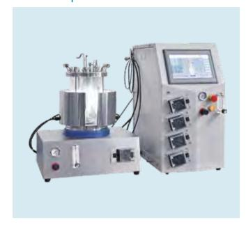
**YC-JGG** is laboratory benchtop illumination bioreactor. The lampshade surrounds the glass vessel without taking up extra space, and is more suitable for plant cell growth.
