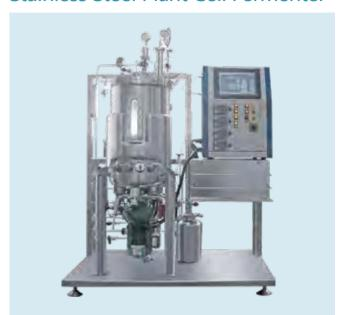
YC-JS is an in-situ sterilized fermenter for microbial culture, with stainless steel as the main body, and suitable for pilot and production.
