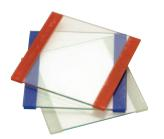
Combs and spacers are injection moulded for consistency and 'clean' well formation.
