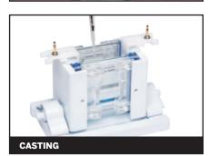
Casting and running – dual purpose PAGE inserts eliminate time- consuming transfer of glass plates between separate casting and running modules. Cam-Pin caster locks PAGE insert onto the ultra-soft silicone mat within casting base to provide a leak-free seal.
