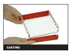
'Plug-and-Go' casting – moulded casting dams clip easily onto the ends of the gel tray for rapid external casting, allowing the multiSUB™ unit to remain in use for gel running.
