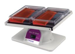
These gel staining / blotting boxes are available in 4 sizes and are the ideal accessory for incubating blots or staining gels.
