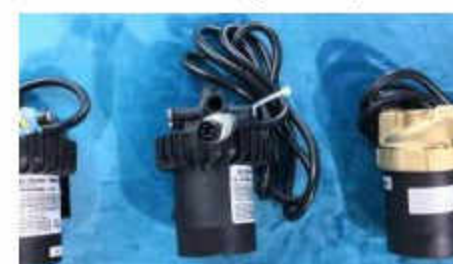
△ Circulating water pump
