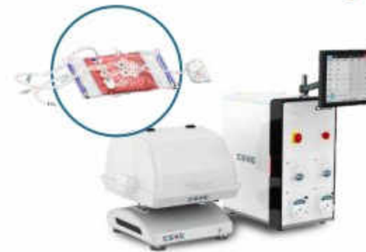
5L culture bag grows for 5-7 days and digest, then inoculate it into 1-3 per 50L fabric carrier bags
