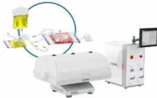
50L culture bag grows for 5-7 days and digest, then harvests (1-1.5) \times 10^{11} cells, therefore can inoculate multiple 200L fabric carrier bags or bioreactors, inoculation density is 6 \times 10^5 cells/ml
