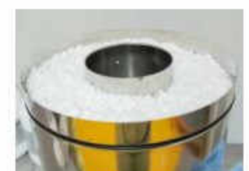
Packed-bed basket impeller with fabric carrier
