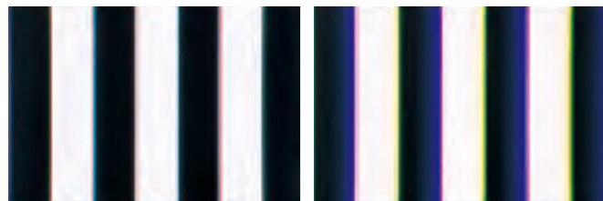
Image where chromatic aberration has been corrected in the SMZ1500 Image that exhibits chromatic aberration Comparison of chromatic aberrations
