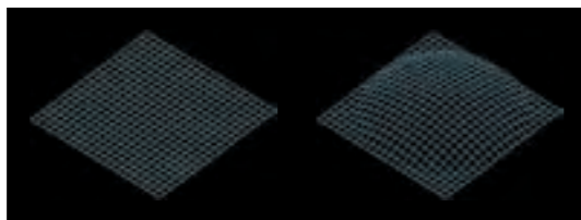
Distortion causes a globular effect as shown above even when you actually observe a flat object.
