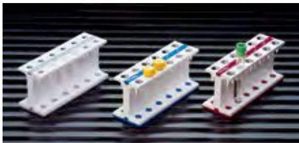
MagneSphere® Technology Magnetic Separation Stand (twelve-position) (Cat.# Z5341, Z5342, Z5343).
