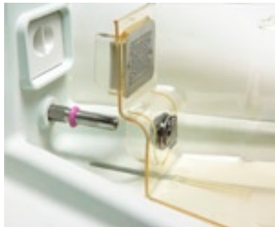
Fixed rack-mounted Edstrom valve (SE Lab valve similar)
