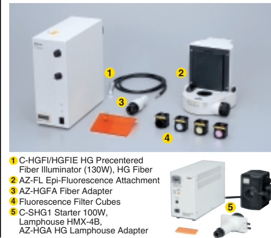
Epi-fluorescence configuration
